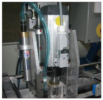
ODM's high speed drill station in the new Super Sewer™ XXL utilizes two Vortec Thread Guard™ needle coolers. One for predrilling and one for sewing in order to maximize production and performance in producing up to 400 sewn book blocks per hour.
