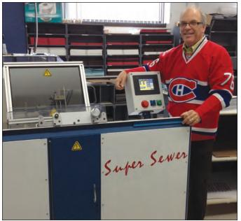
Super Sewer™ side sews book blocks up to half inch thick at 600 per hour utilizing Vortec's Thread Guard™ needle cooler.
