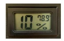
The results were immediate: the enclosure's relative humidity dropped from 55% to 10%, and the temperature stayed between 78 to 82°F (26 to 28°C). Since Jeff installed the first 7715, he has ordered six more to install on Titan's other control panels.
